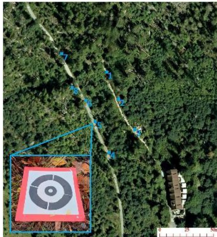
Fig. 6. GCP for UAS photogrammetry Source: Own elaboration
