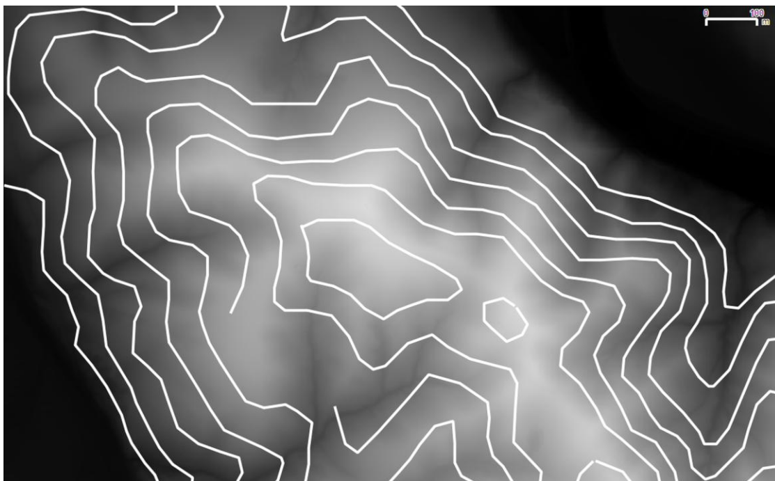
Fig. 9. Comparison of contour lines obtained from WIG map to accurate model Source: own study
