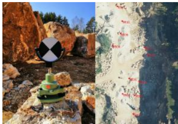
Fig. 1. GCP for TLS surveying Source: Own elaboration
