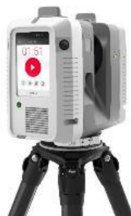
Fig. 3. Terrestrial laser scanner Leica RTC 360 Source: Geotech s.r.o., 2023
